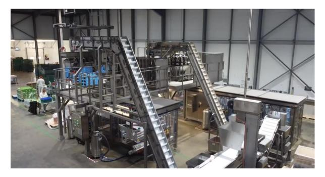
The height and size of the platform, in addition to the location of the support legs, meant careful consideration also had to be given to minimising vibration, as excessive vibration on the platform would impact the performance of the multihead weigher. Specifically, vibrations on the platform would reduce the accuracy of the weigher, increasing product giveaway in the pouches.
