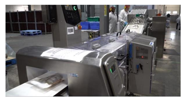
Any non-conforming products are rejected into lockable bins where they are inspected by the quality control team.
