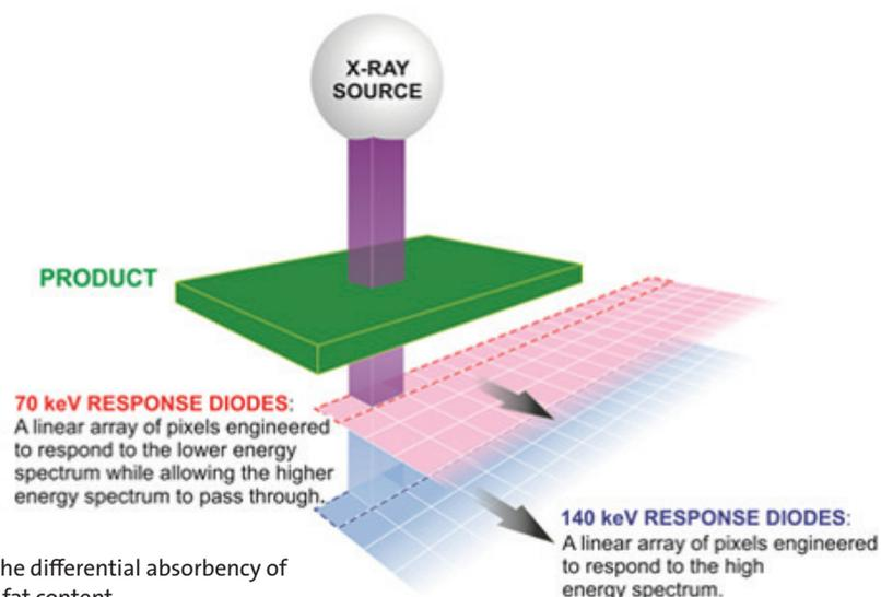
Figure 1: DEXA works by measuring the differential absorbency of two x-ray energy spectra to measure fat content
