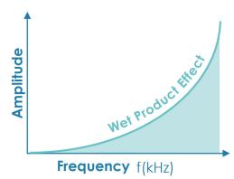
Among other factors, Product Effect interference increases with higher inspection frequencies, which are typically used to detect smaller particles of stainless steel and non-ferrous metals
