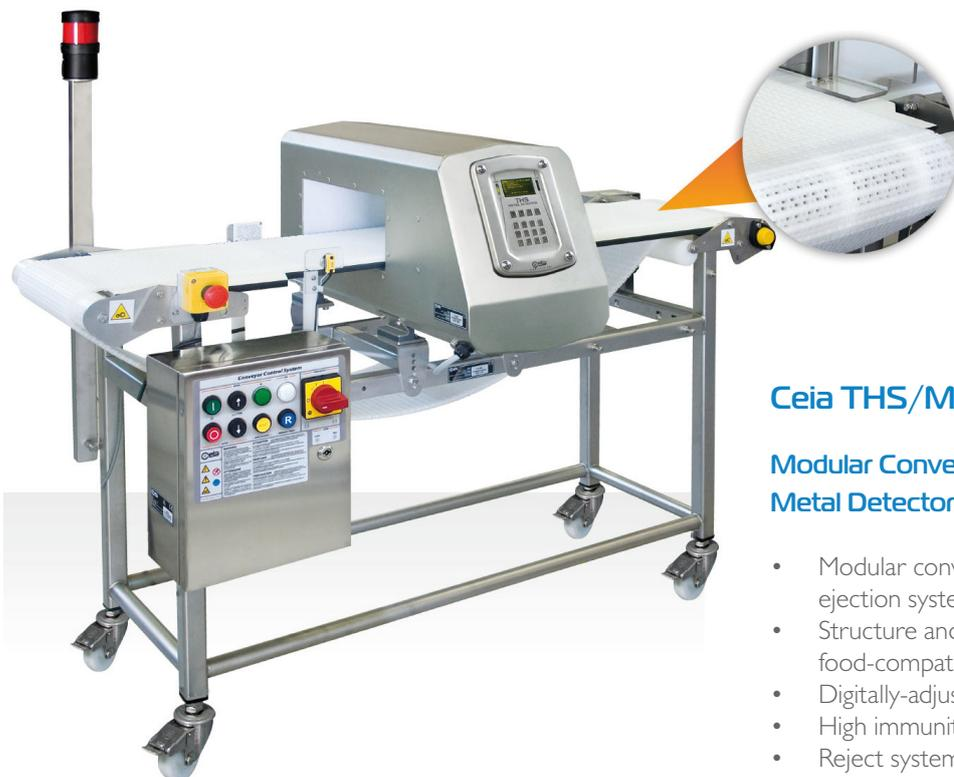
**Structure and components in AISI 304 stainless steel and food-compatible plastic parts**
