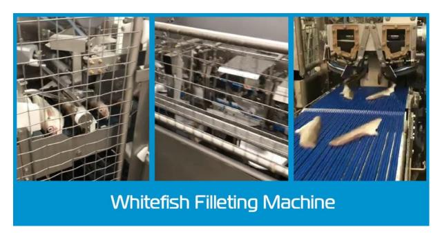
J-cuts are also possible with this machine. In fact, this is the only machine on the market that produces a J-cut for pin boneless fillets as well as standard fillets.
