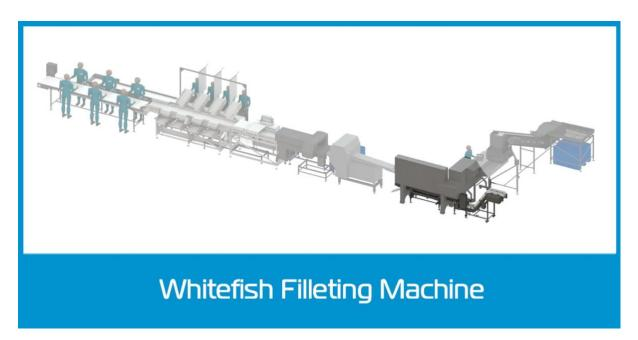
The fish fed into the filleting machine in a process that requires two operators. The filleting machine is specially design for filleting small whitefish – fish that are between 27 and 52 cm and between 300 and 900 grams. This machine is manufactured by one of the world's leading food processing equipment manufacturers and requires just two people to operate.
