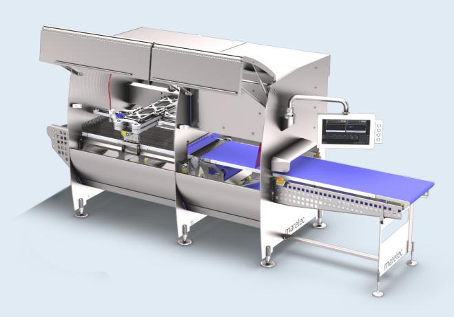
The PORTIO JET is built in a modular way. It starts with the base module where all electronics, scanning and HMI are integrated. As a standard this base unit is controlling a module with 2 cutting stations. This combination is called PORTIO JET 2.
