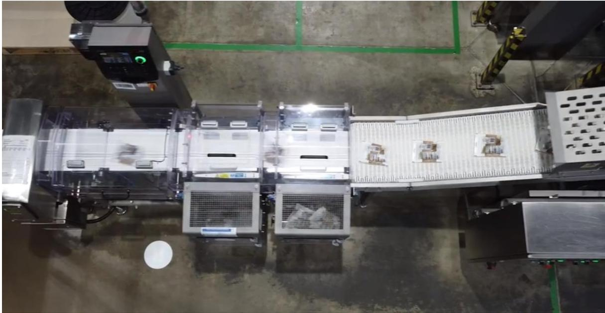
Conforming products continue through to a recirculating packing station that allows operators on both sides ergonomic access to the products for the filling of boxes. The boxes are pushed onto a takeaway conveyor where they are sealed, and a label is automatically applied before palletising.
