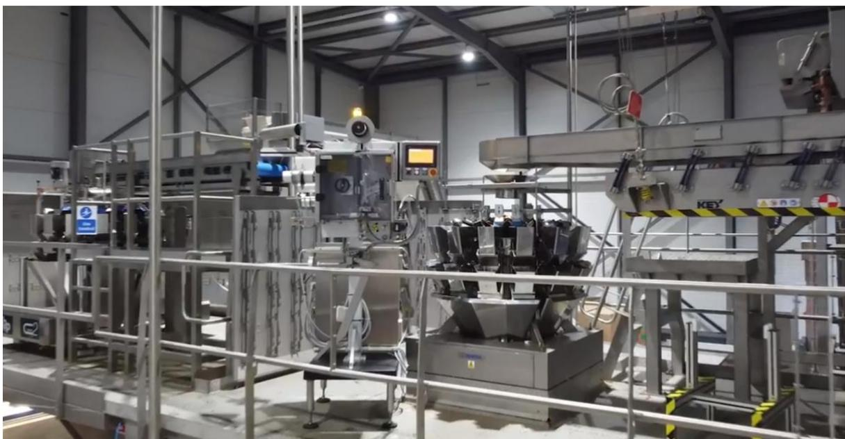
To ensure the platforms were optimised for the process, we conducted a structural evaluation of the platform to ensure any vibrations affecting the multihead weigher were eliminated to guarantee weigher accuracy.
