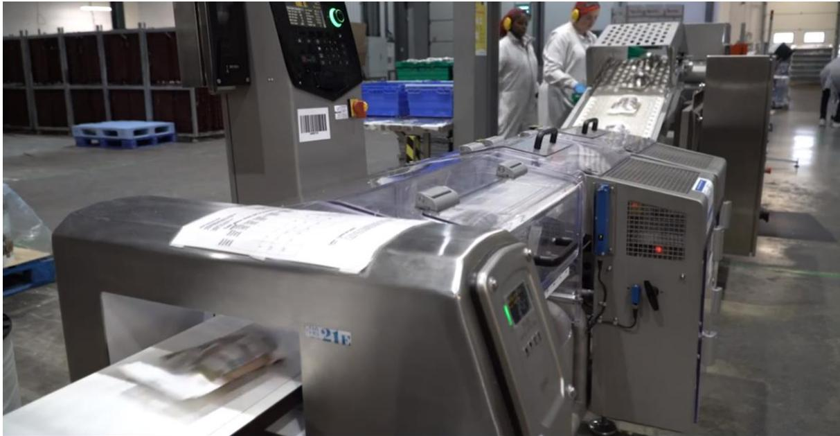
Any non-conforming products are rejected into lockable bins where they are inspected by the quality control team.
