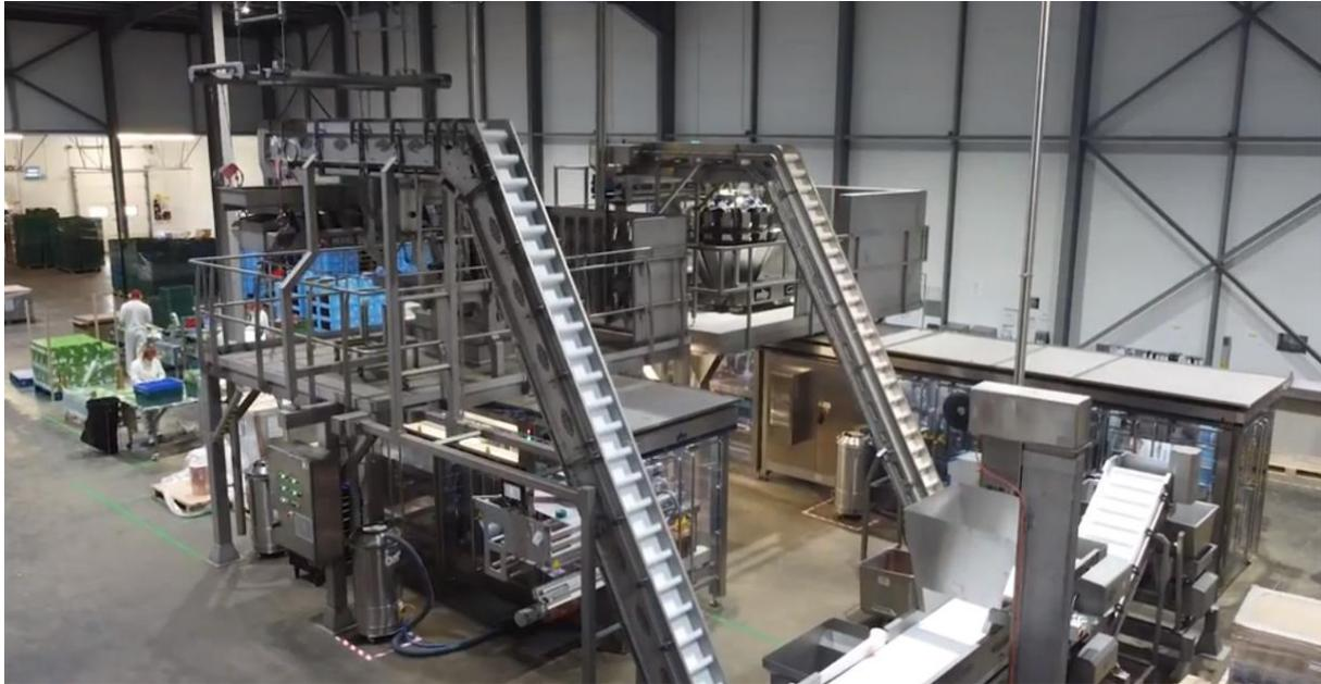
The height and size of the platform, in addition to the location of the support legs, meant careful consideration also had to be given to minimising vibration, as excessive vibration on the platform would impact the performance of the multihead weigher. Specifically, vibrations on the platform would reduce the accuracy of the weigher, increasing product giveaway in the pouches.
