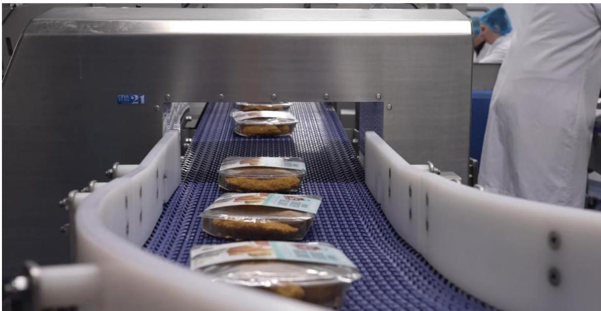
The filled cartons are then placed onto a conveyor that takes the cartons to a case taper and an Ishida carton checkweigher. Data from the checkweigher is exported to the factory's ERP system which then creates the label information. This information is laser jet printed onto the carton before it is delivered to the operator for palletisation. Cartons that are outside the weight tolerance are rejected prior to the label application.
