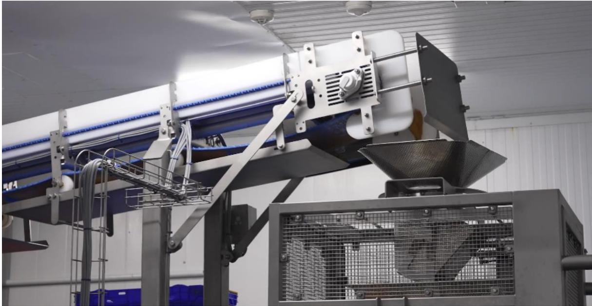
On the new tray packing line, one of the Ishida multihead weighers drops the target weights onto a flighted conveyor that indexes the product into a distribution system located in the retail packing area.
