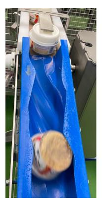
The new bespoke yogurt pot clipping machine was fully tested, refined, and optimised at our facility before being sent to the customer's production line for installation and commissioning.
