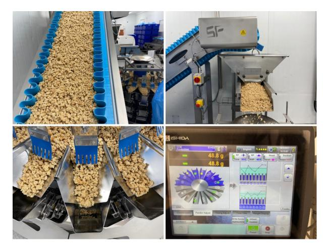
The new weighing system enables the customer to guarantee the target weight at an increased level of throughput. It also automated the process and greatly reduced the need for operators on this part of the line.
